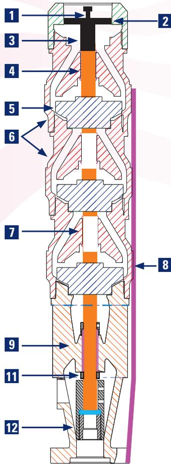
1. Discharge - Optimized for high, efficient production.
